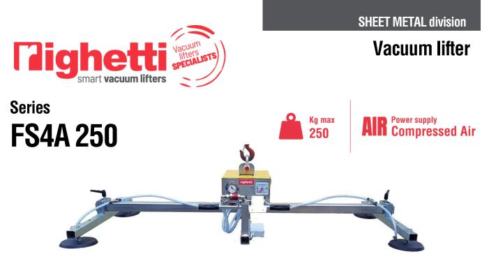
The Vacuum Lifter for sheets metal **FS4A 250** is a model with compressed air operating system and requires connection to the pneumatic system . The model FS4A 250 has a maximum capacity of 250 kg and **4 suction pads** distributed on 2 cross-arms. The pads, equipped with springs, are made of **special oil-resistant vulcanized rubber**, specific for sheet metal.
