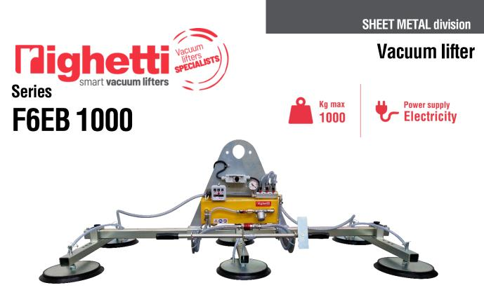
The Vacuum Lifter for metal sheet F6EB is a model with **electric operating system**, it's possible to choose between 400V three-phase or 220V single-phase. The model F6EB 1000 has a maximum capacity of 1000 kg and **6 suction pads** distributed on 3 cross-arms. The pads, equipped with springs, are made of **special oil-resistant vulcanized rubber**, specific for sheet metal.
