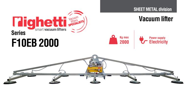
The Vacuum Lifter for sheet metal F10EB is a model with **electric operating system** 400V three-phase or 220V single-phase. The model F10EB 2000 has a maximum capacity of 2000 kg, it has a cross-beam which can be made with different lengths, on standard models L3000 mm, L4000 mm or L5000mm and it has 10 suction pads distributed on 5 arms. The pads, equipped with springs, are specific for sheet metal made in **special oil-resistant vulcanized rubber**.
