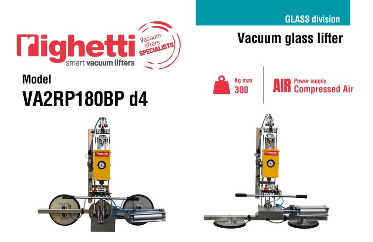
VA2RP180BP d4 is a **pneumatic vacuum glass lifter specific for indoor use**, with two suction pads d. 390 mm and working load limit up to 300Kg. The pads are replaceable along the beam in different positions. The standard central beam is 1500mm long, on request different lengths.
