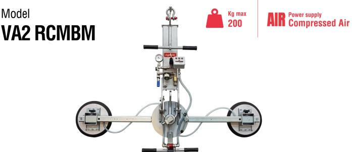
The model VA2 RCMBM is a **vacuum glass lifter specific for indoor use**, with two suction pads d. 310 mm, compressed air powered with lifting capacity up to 200Kg. The pads are replaceable along the arms in different positions.
