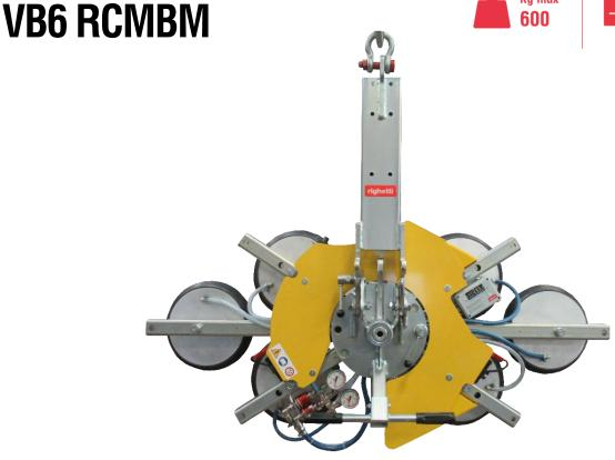
The VB6 RCMBM is a vacuum glass lifter with manual 360° continuous rotation and manual tilting system 0-90°. It has 6 round pads d. 310mm. The pad spread dimension is mm 1420 x 678.
