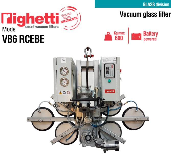
The VB6 RCEBE is a vacuum glass lifter with **electric 360° continuous rotation** and **electric tilting system** 0-90°. It has 6 round pads d. 310mm and the pad spread dimension is mm 1420 x 678.
