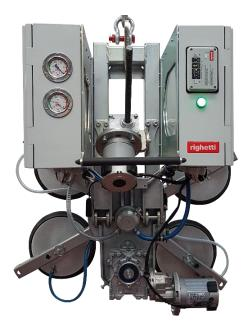
The VB4 RCEBE is a battery-powered vacuum lifter with **continuous 360° electric rotation and powered tilt**. The rechargeable batteries can be easily removed and quickly replaced. The suction pads can be positioned in two different positions or in the PRO version, in four
