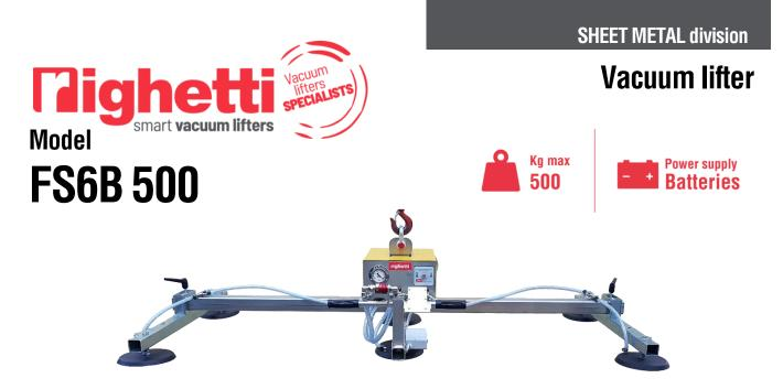
The sheet metal vacuum lifter FS6B is battery powered by high capacity rechargeable batteries (battery charger is included). FS6B has a maximum capacity of 500 kg and **6 suction pads** distributed on 3 cross-arms. The pads, equipped with springs, are made of **special oil-resistant vulcanized rubber**, specific for sheet metal.
