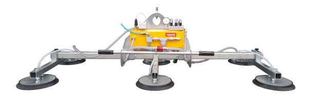
The Vacuum Lifter for sheets metal **F6A 1000** is a model with compressed air operating system and requires connection to the pneumatic system. The model F6A 1000 has a maximum capacity of 1000 kg and **6 suction pads** distributed on 3 cross-arms. The pads, equipped with springs, are made of **special oil-resistant vulcanized rubber**, specific for sheet metal. The lifter can be produced with different crossbeam lengths, from L1500 mm to L4000 mm (different lengths on request).
